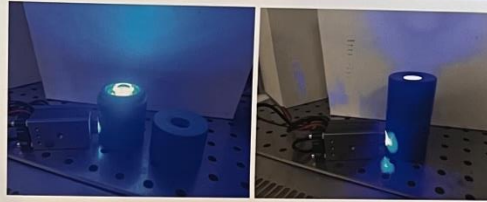
Figure 1: Extremely simple equipment used for LASER-assisted radiolabelling: LASER, standard lead shielded containers for vials with a drill hole and the MAA kit vial
