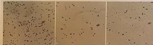
Figure 3: Comparison [^{68}\text{Ga}]\text{Ga-MAA} 25°C (a), LASER (b) and 75°C (c) radiolabelling in Burker chamber
